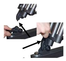
In order to mount the tripod, you must remove the rubber feet till the tripods pointed inner feet are exposed. You will notice on the dolly a little spot which that pointed foot will sit within. Once you have them lined up and set, you must pull the large rubber section of the dolly leg upwards and over the lip, tightening it down.
