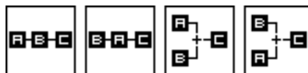
Figure 21: The four topologies in which the effects can be applied after the Amp module of the two module rows; A = Chorus module, B = Delay module and C = Reverb module.
