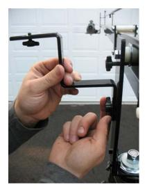
**7.** Attach the monitor mount if using a small LCD monitor. The supplied 12' RCA monitor cable can be used to connect the camera to the monitor. A simple way to deal with the cable is to weave or wrap it on the fixed tilt control rod.
