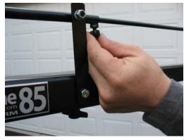
**5.** Now lock the extension with the tightening screw. Once you have squared up the tilt control fixed rod support (2 on the 121), tilt handle and camera mount idler arm; lock into place with the tightening screw (2 on the 121). The camera mount can be set at angles other than 90 degrees for accentuated camera tilting action. Experimenting with different positions will be useful.
