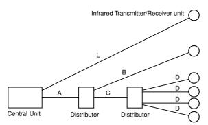
If two or more Infrared Transmitter/Receiver units with different connection cable lengths receive infrared signals from the Chairman and Delegate units, the signal reception level may decrease to cause malfunction.
