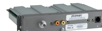
Digital Tuner Card with Pro:Idiom IMP-1500 For 11 Series Hospitality Models and 42- 103-inch Professional Displays
