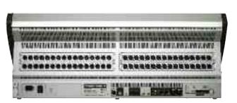
The Vi1 rear panel features 32 mic/line inputs, plus AES (4 channels) and SPDIF (2 channels) digital inputs. A Studer D21m system-based double card slot accommodates a range of I/O options including AES and MADI, which can be used to connect the standard 64 channel Vi Series Stagebox, with all inputs and outputs fully patchable from the Vi1 control surface.
