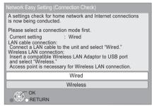
If "Wireless LAN Adaptor is not connected." is displayed, check that the Wireless LAN Adaptor is fully inserted. Alternatively, disconnect and reconnect it. If there is still no change in the display, consult your dealer.
