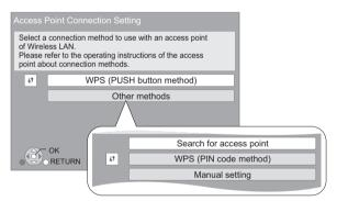
WPS (Wi-Fi Protected Setup) is a function that facilitates settings relating to the connection and security of wireless LAN devices. To see whether your Wireless router (Access point) supports WPS, check the Wireless router operating instructions.
