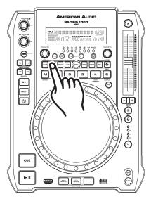
**ECHO EFFECT:** The Echo effect adds an echo to your output signal. The Echo effect has two adjustable parameters, Parameter Time (PT) and Parameter Ratio (PR). The PT will adjust the Time Range and The PR will adjust the Frequency Range (see "Parameters" in the next section).
