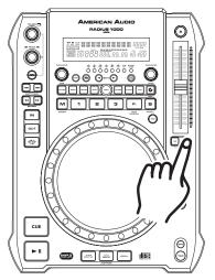
Holding down or tapping on the (-) PITCH BEND BUTTON (5) will provide a slow down in the playback pitch.
