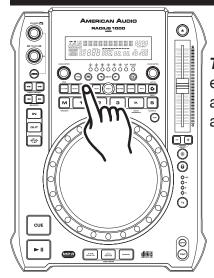
**TRANS EFFECT:** The Trans effect simulates a real-time mixer transformer effect. The Trans effect has two adjustable parameters, Parameter Time and Parameter Ratio. The PT will adjust the Trans Speed and The PR will adjust the Trans Audio Length.
