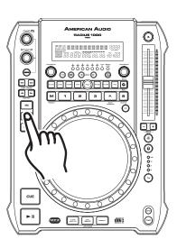
**REPLAY LOOP** - The *RELOOP* (15) function allows you to return to your stored loop at any time. The *IN BUTTON* (15) and *OUT BUTTON* (15) LEDs will indicate a loop is stored in memory, and may be played at any time. To replay the loop, press the *RELOOP BUTTON* (15). The *IN BUTTON* (15) and *OUT BUTTON* (15) LEDs will again begin to flash indicating SEAMLESS LOOP mode has been activated and your stored loop will immediately begin to play.
