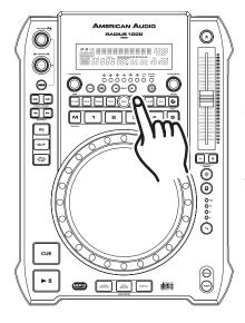
**PHASE EFFECT:** The Phase effect tweaks the original sound to add different tonal definition. The Phase Effect has two adjustable parameters, Parameter Time (PT) and Parameter Ratio (PR). The PT will adjust the Time Range and The PR will adjust the Frequency Range (see "Parameters" in the next section).
