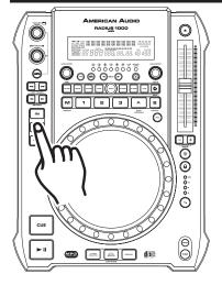
3) Press the *OUT BUTTON* (15) to set the ending point for your SEAMLESS LOOP (Figure 20). The *IN BUTTON* (15) and *OUT BUTTON* (15) LEDs will immediately begin to flash rapidly, indicating the SEAMLESS LOOP mode has been activated.
