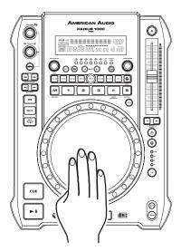
**IN CUE MODE:** While in cue mode and when the touch sensitivity function is active, tapping on the *JOG WHEEL* (9) can be used to start playback. The unit will continue to playback until the *JOG WHEEL* (9) is released. Once the *JOG WHEEL* (9) is released the unit will return to the last cue point.
