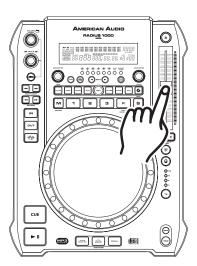
**Using the Pitch slider (3):** Be sure the pitch function has been activated as described above. To use the *PITCH SLIDER (3)* slide the slider up and down. Down will increase the pitch and up will decrease the pitch.
