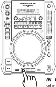
**ACTIVATING TOUCH SENSITIVITY:** Before you can use the *JOG WHEEL* (9) to control the play and cue commands you must first activate the jog wheel touch sensitivity. To activate the touch sensitivity mode, press the *A.CUE SCRATCH BUTTON* (12). This will activate touch sensitivity mode.
