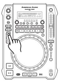
2) Press the *IN BUTTON* (15). This will set the starting point of the SEAMLESS LOOP. The *IN BUTTON* (15) LED will flash then glow.
