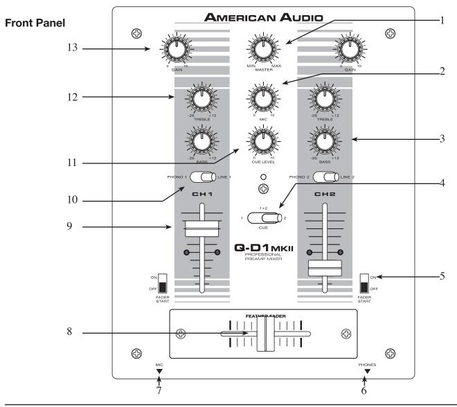
**1. MASTER VOLUME CONTROL -** This rotary knob is used to control the master output level (volume). To avoid distorted output try to maintain an average output signal level +4 dB. Be sure this volume control is always set to zero before turning the unit on.
