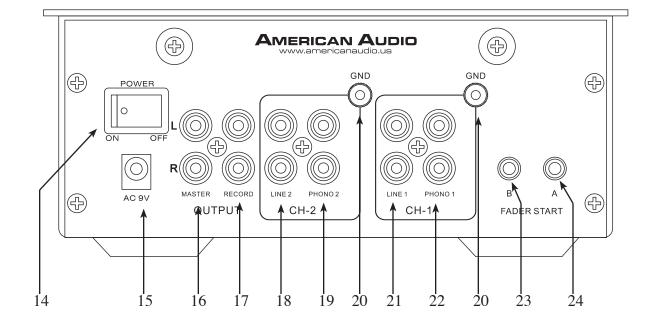
**14. MAIN POWER SWITCH** - This is the main power ON/OFF button. Before main power is applied, be sure you have made all connections to the mixer. Also be sure your amplifier(s) is tuned off. Remember to avoid damaging pops, mixer on first and turned off last.
