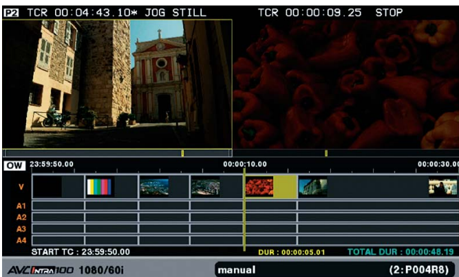
Playlist preparation example 2: Displaying player side and recorder side playback screens (with the player side selected)
