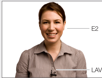
Countryman E2 and typical cardioid lavalier on the chest, approximately gain matched for the voice band at the mix board.
