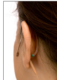
The E2 is unaffected by head position; directional lavs change their gain and frequency response.
