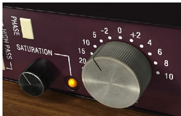
The Phase switch, Saturation knob and indicator LED and the Output Volume.
