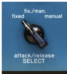
Figure 2: Attack and release times are constant in the FIXED position and cannot be changed. In the other two settings you can use the Attack and Release knobs to set the times.
