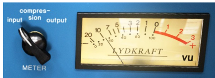
Figure 1: Use the Meter knob to select what the VU meter displays.
