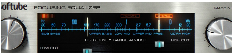
Figure 3: From left to right, top to bottom: saturation meter, remote control indicator (Pro Tools only), and stereo indicator. The selected frequency range is indicated by the yellow needles.
