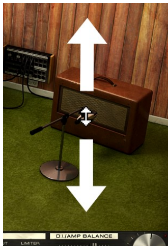
Figure 2: Click-and-drag up or down to change microphone position. Move the mouse up to first move the mic closer to the cabinet, and then to the off-axis position.
