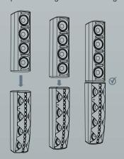
**CBT 70JE EXTENSION CABINET** The CBT 70JE further extends the pattern control of the CBT 70J by doubling its height. This lowers the frequency to which the speaker holds a consistent coverage pattern. The 70JE also extends the low frequency capability of the system.
