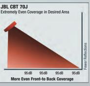
**HIGH OUTPUT & WIDE BANDWIDTH** The two-way CBT 70J produces high sound levels, rivaling larger two-way loudspeakers in output sound level as well as providing wide, smooth frequency response throughout its coverage area.
