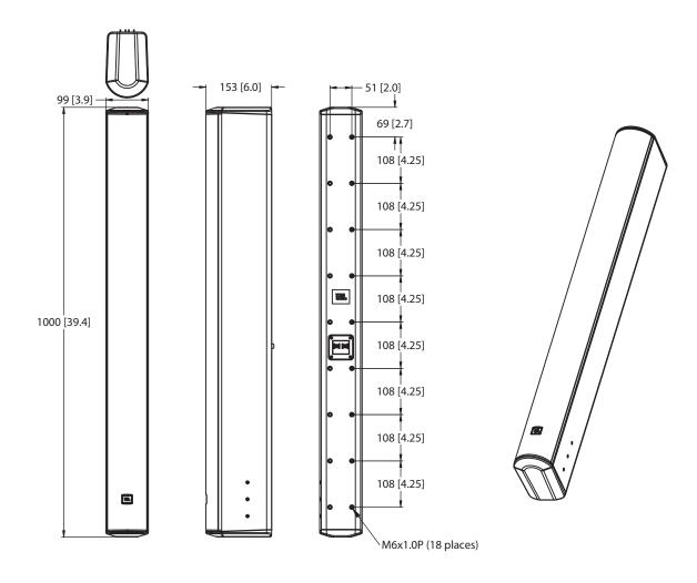
CBT 100LA Line Array Column Loudspeaker with Sixteen 50 mm (2 in) Drivers
