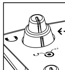
*Effects return is located under the headphone volume on each SoleMix section of the JamHub's main unit. It's also its own knob on the SoleMix remote.*
