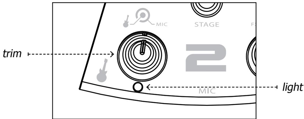
1. Use the double knob called "trim" to set your input gain (note: you don't need to put on headphones to do this step). Use the light under the dual trim knobs to get this right.
