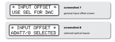
To change selected optical inputs, scroll through the following menu by pressing the OPTICAL input switch repeatedly:
