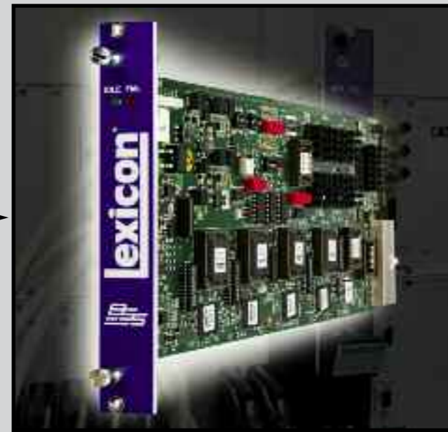
The Soundcraft Vi Series™ Processor Card plugs into the local rack to add world-renowned Lexicon and BSS processing to the Soundcraft Vi digital mixing platform.
