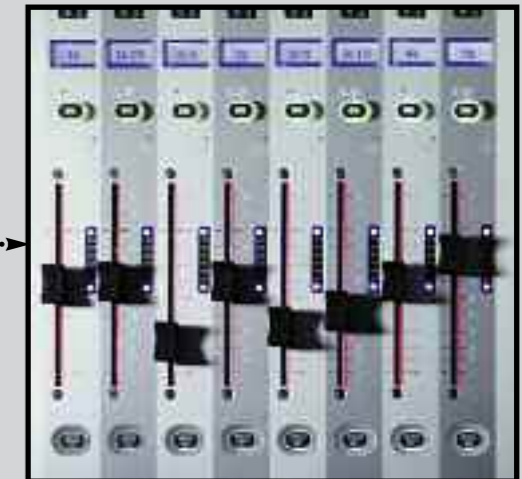
Bringing up the output channel strip and touching the Graphic EQ button immediately assigns the first 30 faders on the console to Graphic EQ, with the Soundcraft FaderGlow™ changing to red, indicating that the console is no longer in channel fader mode.
