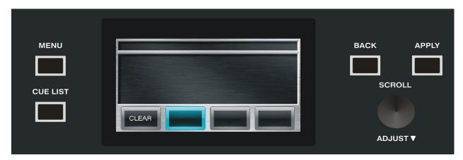
The default display, after the power-up is completed, is the Menu as shown below.
