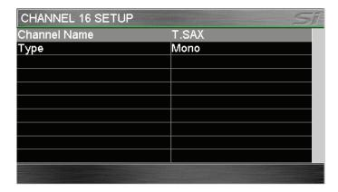
Select the required channel by pressing its SEL button. The channel's name and type (mono or linked) can be edited/set. When a channel is linked it is automatically linked with an adjacent channel such that the left-most channel is an odd-numbered one and its right-hand twin is an even-numbered one. The FaderGlow<sup>TM</sup> bars are illuminated white for linked channels.
