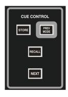
In the CUE CONTROL section down near the center section masters, press the STORE button. If no cues have been stored, your settings will be saved in CUE 001, labelled Snapshot 1 (which you can re-name at any time.
