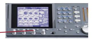
4. Turn the POD 4 knob (the fourth knob under the display) to select the mic/line inputs (labeled M/L).
