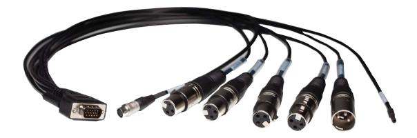
The XL-88 Breakout Cable is an optional accessory for the 788T/788T-SSD Digital Recorders. It securely connects to the 788T's rear panel Multi-Function DE-15 connector. The cable breaks out into four balanced female XLR connectors for AES Inputs 1-8, a balanced XLR male connector for AES Out 5 and 6, a 4-pin Hirose female connector for 10-18 VDC input, and a bare wire sealed with a heat shrink for Logic In and Out.
