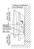
Note: As a force of approx. 18 kg (39.68 li is applied to the speaker receptacle at the time of speaker installation, attach it in a location durable enough to withstand the force.
