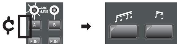
fU Adjust an input level volume on the front part properly and then press the chime button.
