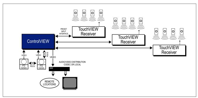
Figure 3 – TouchVIEW setup, expanded.
