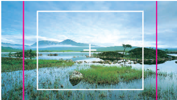
Screen Size: 16:9, Aspect Mode: 4:3 Aspect Marker Color: Magenta, Marker Bright: 90IRE, Width: THICK,
