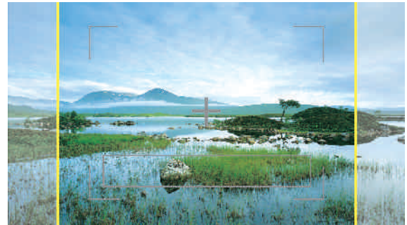
Screen Size: 16:9, Aspect Mode: 4:3, Aspect Marker Color: Yellow, Marker Bright: 40IRE, Width: THIN,
