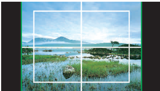
Screen Size: 16:9, Aspect Mode: 4:3, Aspect Marker Color: Green, Marker Bright: 90IRE, Width: THICK,
