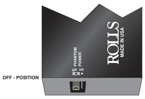
Rolls utilizes a way of switching phantom power ON and OFF thru a three pin jumper wire that is attached to the unit and a external bridge clip to act as a switch for switching between two preset unit options. For example on other Rolls units it might be for switching between phantom power on/off as illustrated above or it may be used for switching between ground/lift or other options as denoted on the silk screening of the unit.
