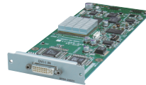
BRSA-20DD1 Input: DVI-I (SXGA, WXGA, XGA) x 1 with frame synchronizer and scan converter
