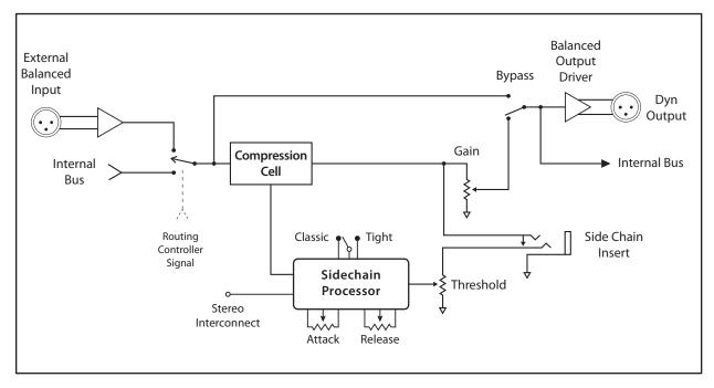
The input to the Dc1 is electronically balanced and directly feeds our unique compression cell. The Side Chain allows for stereo coupling, the insertion of an equalizer, or controlling the gain cell with an external source.
