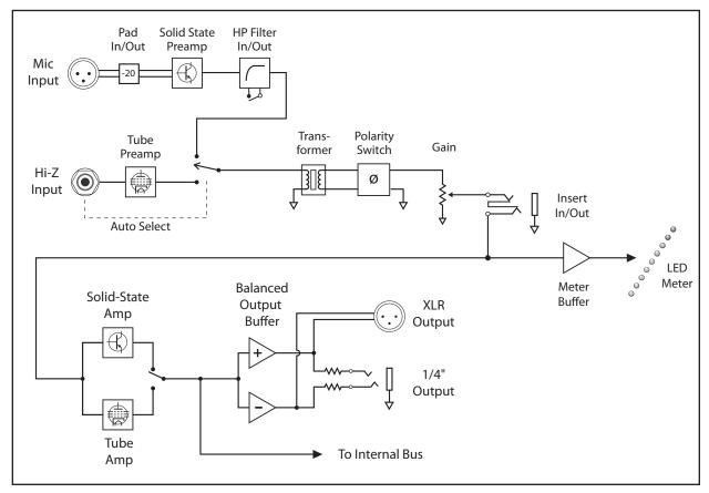
The Mz2 preamplifier is the first stage of Everest. Microphone signals are first preamplified with a discrete transistor stage. Hi-Z instrument signals enter the Mz2 though a high-voltage vacuum tube. Next in line, a Jensen line level transformer isolates the signal before the gain control and insert point. The secondary tube or solid-state preamp allows even more flavor combinations.
