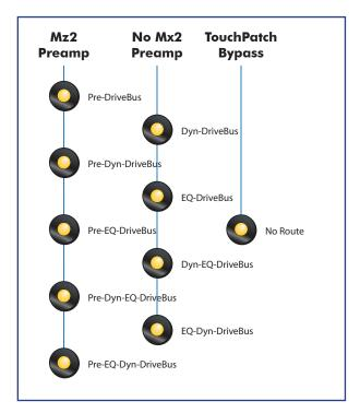
Unique to the ECS-410, the TouchPatch<sup>™</sup> routing allows you to route any section to and from any other section with a touch of a single button. TouchPatch controls what is feeding DriveBus and anything not routed is available to be used individually from the back panel.
