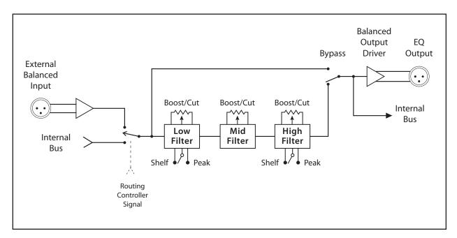
The electronically balanced input stage input goes directly into the passive EQ sections. The low and high bands can switch between peaking and shelving filters. The mid band is a peaking filter.
