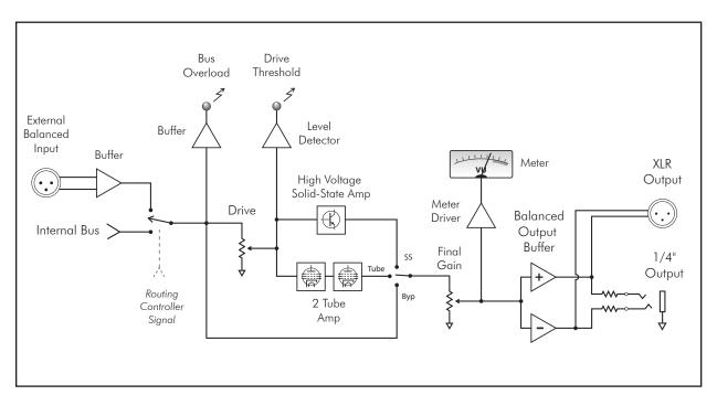
Db2 - Drive Bus Master Output & Drive Section
