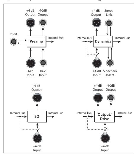
These diagrams show the input and output connections, as well as the input switching when using TouchPatch.
