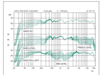
**Figure 2**: The curves above show the effect of the 'bass', 'mid' and 'treble' level controls, and the 'bass tilt' and 'bass roll-off' controls on the free field response, measured at 2 m.
