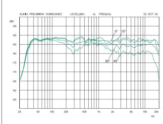
**Figure 1**: The curve group shows the horizontal directivity characteristics of the 1038BC in its vertical configuration measured at 2 m.
