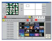
We also offer control software called the HVS-30GUI. This can be installed on any PC and will provide users with full switcher control over IP.
