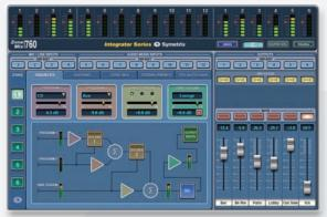
The Zone Mix 760's software application hides nothing more than two mouse clicks away from you. Zone signal flow and priority mixing is built right into the user interface (shown).
