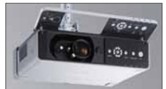
The front panel covers the lens to protect from dust, and conceals the controls to prevent accidental misoperation. It can be opened for easy access to controls even after the projector is mounted to the ceiling.
