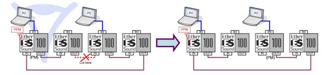
This system is safer than a classic daisy-chain, as a dead link will interrupt audio and data transmission only few ms before recovery. However, you can handle only 64 EtherSound channels, and not 128.
