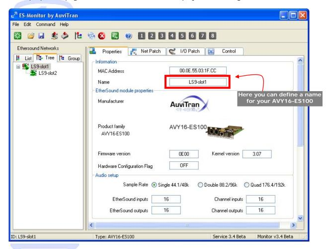
For Audio routing part, AVY16-ES100 is seen by default as a bidirectional EtherSound device with 16 inputs and 16 outputs but could be set as 8 inputs and 8 outputs using the "YGDAI mode" buttons in the Control page.
