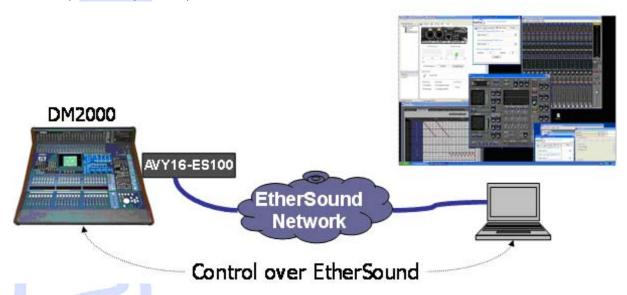
Before using remote control over EtherSound few conditions must be respected:
