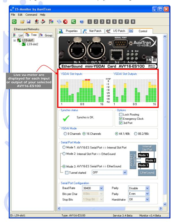
All standard parameters of the AVY16-ES100 can be handled in this control page and you can use the vu-meters to control remotely the audio sent and received by the AVY16-ES100 to your Yamaha device.
