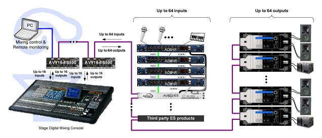
This is the classic Daisy-chain configuration. The computer on which ESMonitor was installed is connected to the "IN Port" of the first device in the network, the primary master (here, an AVY16-ES100). A primary master is the first EtherSound-based device of an EtherSound network which has its "IN Port" not connected to another EtherSound device.
