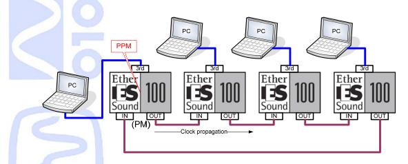
In this configuration, only 64 channels are available, as you must always insert audio downstream, and extract upstream. Loopback is also automatically activated on each device when ring mode is turned on. When a link is broken, the device which has its "In port" open becomes automatically primary master and audio is not interrupted more than few milliseconds.
