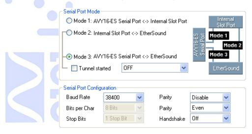
Hardware RS232 tunnelling function enables you to transmit standard RS232 data over EtherSound. This function is very useful to remotely control from a digital mixing console, using only EtherSound connection, a set of AD8HR connected to EtherSound by AVB32-ES or by AVKit-ES for AD8HR. The digital mixers that can manage AD8HR from a remote serial connector are: PM5D, M7CL, LS9, DM2000, DM1000 and DME64N/24N.
