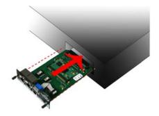
You might need to push your board firmly inside the slot to make sure the connector inside is properly plugged
