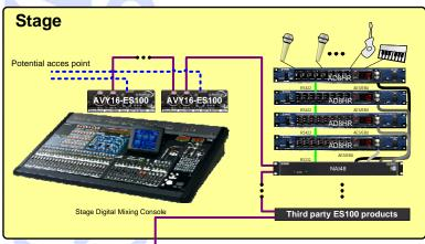
In this configuration, control PC can be plugged on any AVY16-ES100 3rd port. It allows you to monitor the whole network, no matter where you are on stage, and without any architecture modification (e.g. cable disconnecting).
