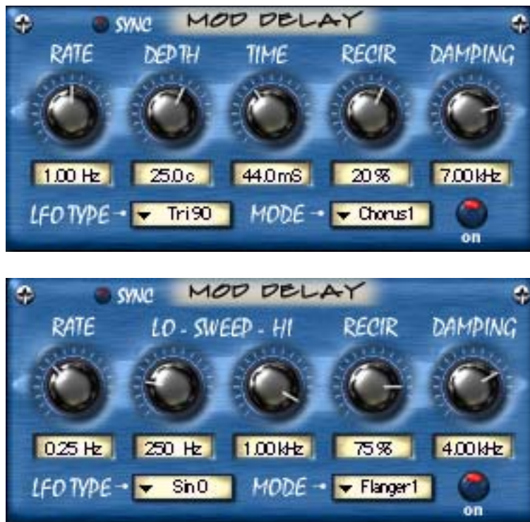
Figure 125. The Mod Delay module The label and function of the second two knobs depend upon the Mode menu selection.
