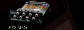
MYS-AD24 8 channel Analog Input Card (24 bit)
