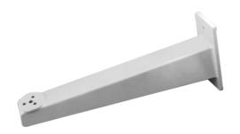
The **PM105** is a medium duty wall mount designed for mounting lightweight pan/tilts and is capable of handling loads up to 40 pounds (18.14 kg). The **PM105** can be used with the PT270P, PT270-24P, and PT280-24P pan/tilts.
