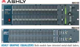
ASHLY GRAPHIC EQUALIZERS Both models have detented metal-shaft faders, precision Wein-Bridge filters, Constant-Q, selectable 15dB or 6dB range, LED level indicators, high-pass filter and level control. Both include XLR, 1/4" balanced and Euroblock I/O.
