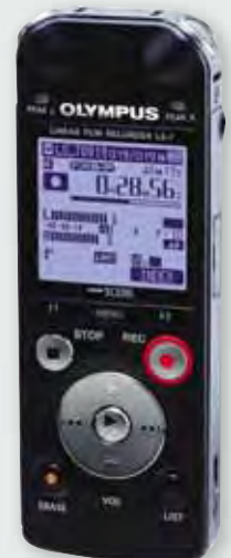
OLYMPUS LS-7 - Linear PCM/MP3/WMA recorder, w/ 4GB of internal flash memory, MicroSDHC slot Page 246
