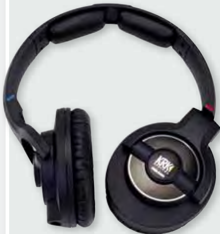
KRK KNS8400 - Dynamic, closed-back headphones, 5Hz-23kHz, 36 ohms Page 96
