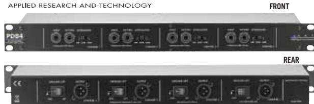
**ART PDB4 FOUR-CHANNEL PASSIVE DIRECT BOX** With four fully transformer-isolated direct boxes in a 1RU chassis, the PDB4 has switchable input attenuation and ground lift on each channel. Input jacks are unbalanced 1/4" TS and output jacks are balanced XLR-M.
