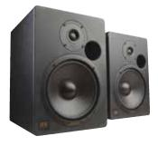
EVENT ELECTRONICS 20/20BAS STUDIO REFERENCE MONITOR This two-way front ported speaker incorporates fully discrete Class AB amplifiers providing up to 80W of program power for the 1" silk dome tweeter and 7.1" woofer. The original transducer design and cabinet volume of the 20/20BAS have been maintained; the high and low frequency amplifiers, cabinet bracing, and overall construction redesigned to improve audio characteristics, increase dynamics and extend reliability.
