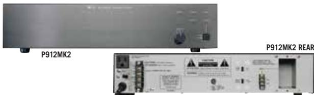
**TOA P-900 SERIES POWER AMPS** These are modular single-channel power amplifiers for paging, background/foreground music distribution and music/messaging-on-hold. All feature one 900 Series input module slot for custom system configuration. All include 25V, 70V and 8Ω transformer-isolated speaker outputs with screw terminal connector and protective cover plate, and a 5-year warranty. Please consult input modules listing for list of available modules.
