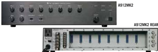
**TOA A900 SERIES MIXER AMPS** These modular mixer/amplifiers are engineered for high performance with wide frequency response, very low noise and distortion, and excellent output regulation. Pre-Out/Power-In jacks allow connection of external signal processing between the mixer and amplifier sections. Come with 8 input module ports, 2 mute circuits, tone controls, remote master level capability, insert point. Please consult input modules listing for list of available modules.
