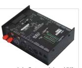
pin-out scanned for continuity as well as proper polarity. Features a balanced 1kHz Test Tone oscillator with a calibrated variable level control. The CS1000 also features phantom power voltage and polarity (both signals present) testing as well.
