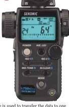
entered manually. After processing, a USB cable is used to transfer the data to one of the Sekonic L-758 meters. Up to 3 camera profiles can be stored in the meter. Any number of profiles can be stored with the software. Once loaded, the Sekonic L-758Cine makes incident and reflected-light spot readings that are precisely tuned to the dynamic range of the profiled camera.
