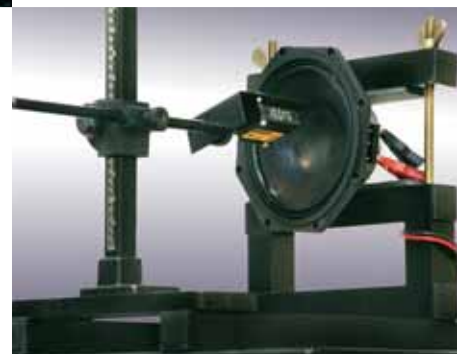
Above: Laser scanning equipment helps evaluate cone transducers such as the neodymium PS8 woofer.
