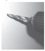
Drill the mounting holes where the marks were made with a pencil. Use a 5/16" concrete drill bit (commercially available).
