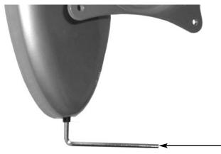
Use the M3 Allen Wrench (supplied) to tighten the locking screw that is located on the bottom of the mount base. This locking screw will prevent the mount and display from being lifted off of the wall plate.
