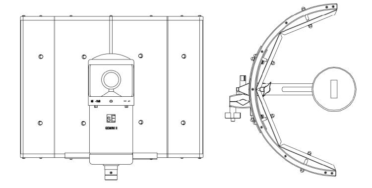
The ideal placement for your microphone is where the mic's capsule is approximately even with the front edge of the RFX, and centered vertically with the filter – but some mics sound better when pushed a little closer, and some a little further away.
