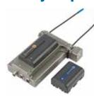
The receiver can be powered with an optional battery "sled" adapter that accepts standard "L" and "M" style rechargeable batteries. The adapter includes an integrated SREXT plate for the rear panel audio outputs. Typical runtime with a 7.2 V, 2200 mA "L" style battery is approx. 11 hours.
