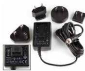
AC power supply with standard C14 inlet and locking LZR coaxial output connector. Interchangeable blades/posts for use in Europe, UK, Australia and USA; 100-240 V, 50/60 Hz input; 12 VDC (regulated), 0.3 A max. output, 6.0 W.
