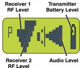
and mode selections. In the ratio diversity mode, the Main Window displays audio levels, transmitter batter
