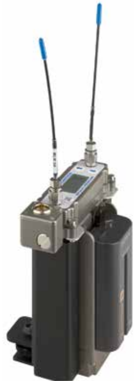
The receiver provides stand-alone operation with the battery sled adapter and mounting sleeve. It can be mounted in any position with Velcro, or in horizontal and vertical positions using the mounting foot, or mounted directly onto a 1/4-20 threaded stud on a tripod.
