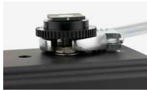
Tighten the jam nut to prevent the foot from rotating
